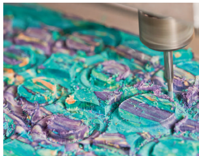
7. Various shapes and sizes are cut out on a CNC machine.
